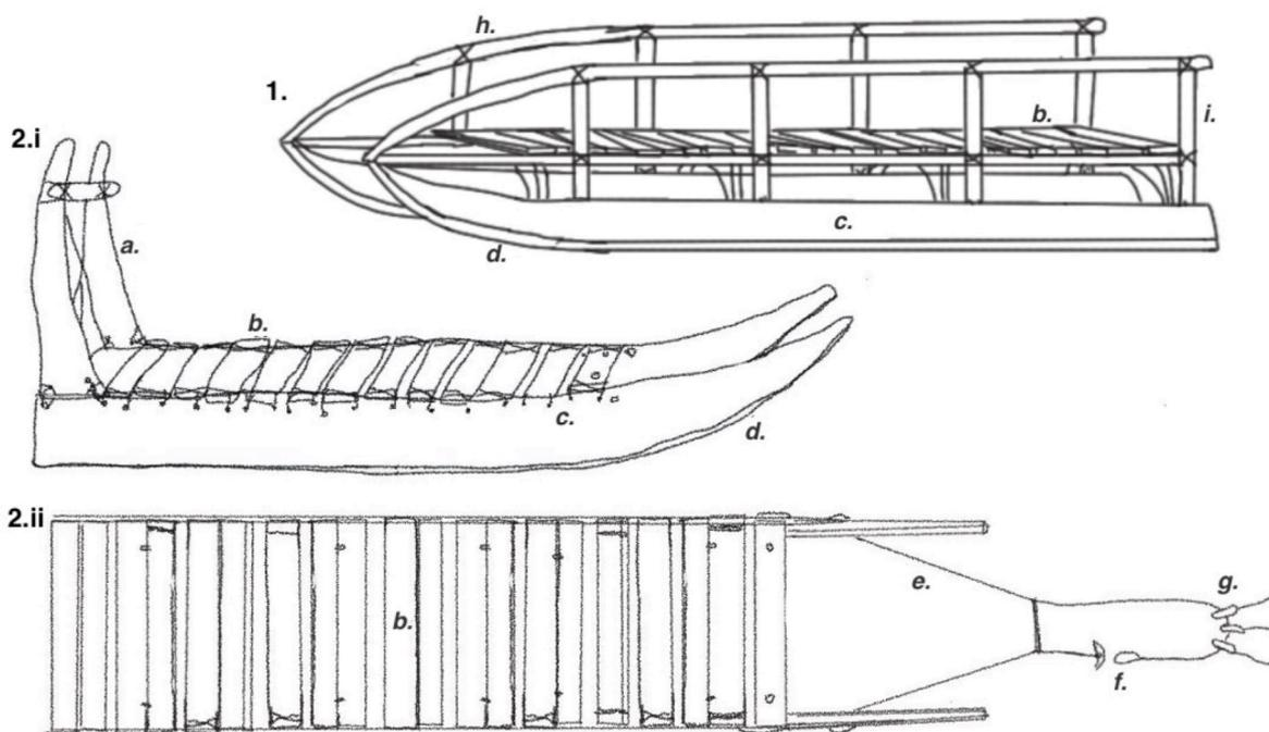
Fig. 1. Terminology of components of the built-up (1) and the low (2) dog sleds. a. Upstanders, b. Cross-pieces, c. Runners, d. Sled shoeing, e. Front strap/trace, f. Clasp, g. Buckles to attach the traces for the dog's harness, h. Rails, i. Stanchions. Types are based on those in Murdoch (1892) and Holtved (1967). Illustration by Emma Vitale.
